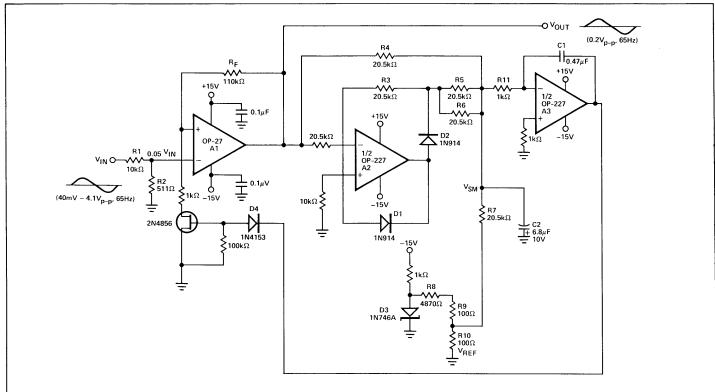
In this circuit, a JFET transistor is used to control the gain of the low-noise OP-27 amplifier over a two-decade input voltage range. For inputs from 40mV to 4.1V peak-to-peak, the AGC maintains a 0.2V peak-to-peak output.
