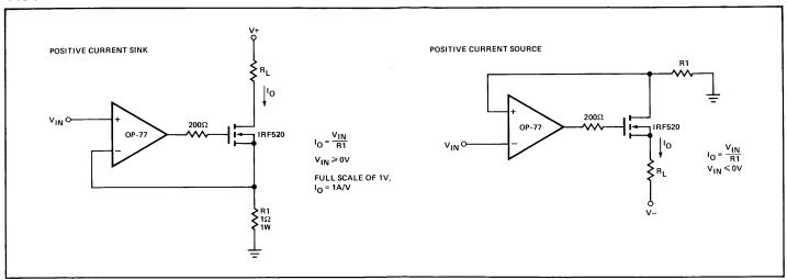
These simple high-current sinks require that the load float between the power supply and the sink. In these circuits, OP-77's high gain, high CMRR, and low  $TCV_{OS}$  assure high accuracy.
