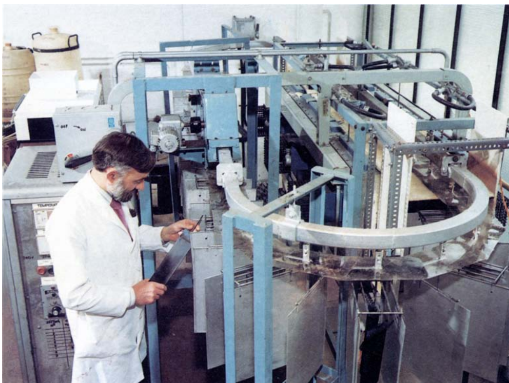
Fig. 3 Laboratory track and tunnel furnace used in the preparation of small electrodes by the paint/thermal decomposition process. The small electrodes are suspended between large heat-conserving baffle plates
